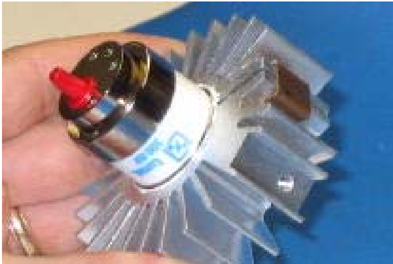
Step 7: Push down until fully seated against heatsink.
