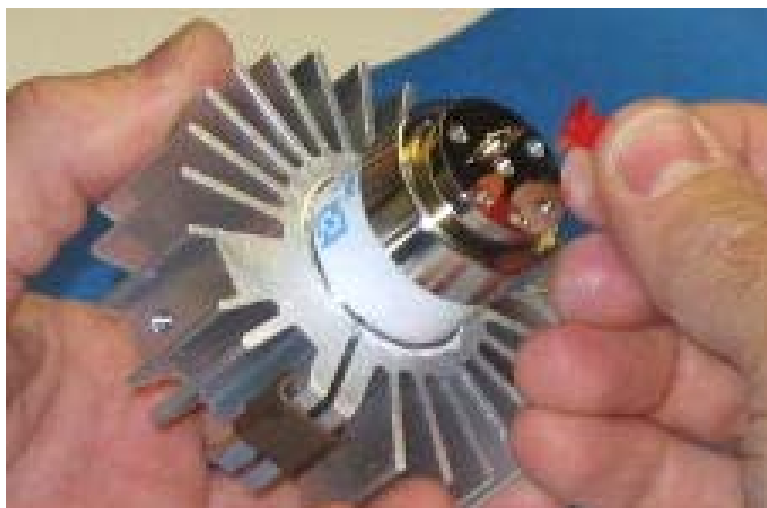
Step 9: Remove the protective cap from the lamp pinch off seal.
